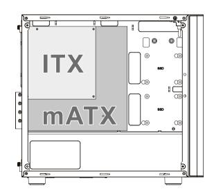
CPU cooler max height: 155mm
