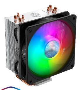
Hyper 212 ARGB is equipped with SickleFlow 120 ARGB fan, providing the best balance between airflow and static pressure for optimal cooling. It features addressable RGB compatible with certified motherboards. Its 4 heat pipes using Direct Contact Technology ensures a smooth contact surface to provide exceptional cooling efficiency.
