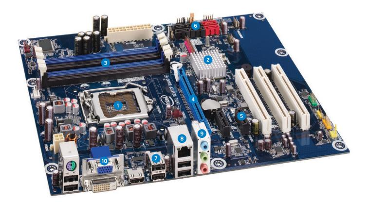
Support for the Intel® Core™ i7 and Intel® Core™ i5 processors in the LGA1156 package, featuring Intel® Turbo Boost Technology<sup>1</sup> and Intel® Hyper-Threading Technology<sup>2</sup> for exceptional performance and scalability
